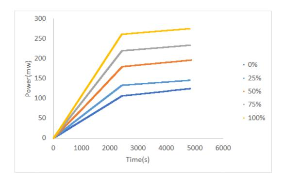
Figure 4.1. Power Consumption for minimum CPU frequency
