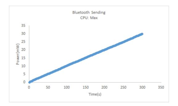
Figure 4.9. Power Consumption for Bluetooth sending
