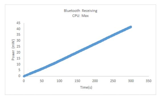
Figure 4.8. Power Consumption for Bluetooth receiving
