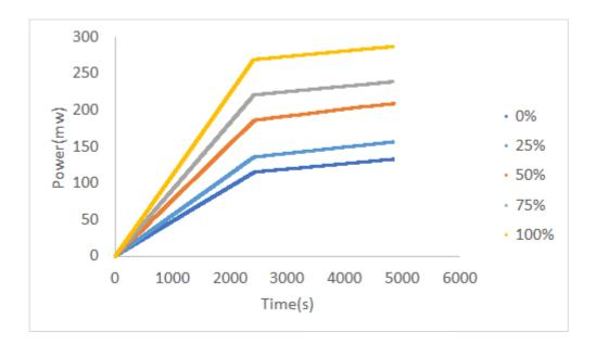
Figure 4.2. Power Consumption for Maximum CPU frequency
