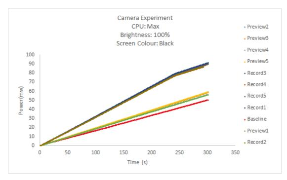
Figure 4.7. Power Consumption for Camera
