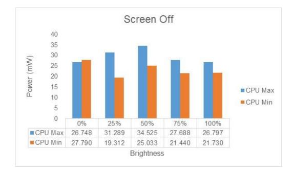
Figure 4.4. Total Power consumption for screen off
