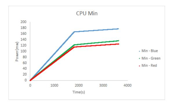
Figure 4.6. Total Power consumption for different color in max CPU Frequency
