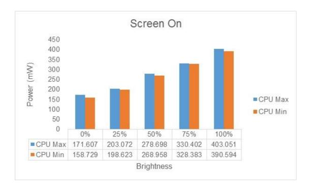
Figure 4.3. Total Power consumption for screen on
