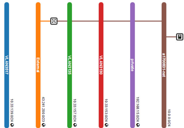
Figure 10: The network topology of OpenStack web server. Each colour represents a sub-net, and sub-nets cannot communicate with each other by default. The icon between “External” sub-net and “a1700831-net” sub-net represents a router, and the icon under “a1700831-net” sub-net is our web server.
