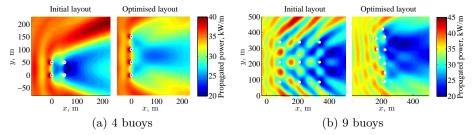
Fig. 8: The wave field around the 4 and 9-unit arrays of WECs with the initial (left) and optimised (right) layouts. White circles show the location of submerged spherical buoys. The wave propagates from left.
