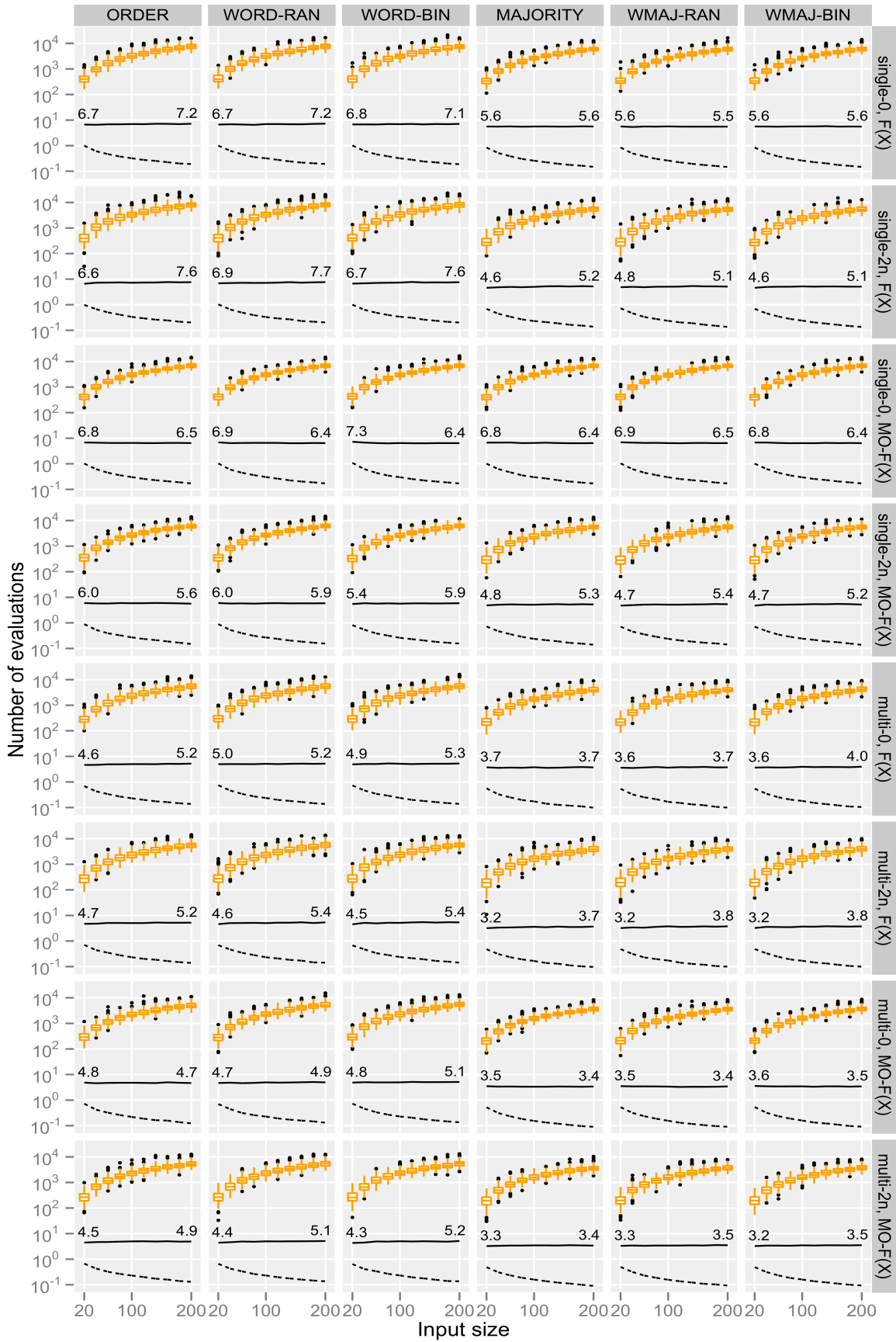
Figure 4.1: Number of evaluations required by (1+1)-GP until the individual X_{max} with maximum fitness is found, shown as box plots. The solid line is the median of the number of evaluations divided by n \log n , the dashed line is the same median divided by n^2 .
