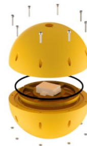
Figure 2. Buoy assembly (0.136m diameter sphere)
