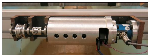
Figure 3. PTO assembly (from left to right: rope spool, shaft coupling, motor-encoder-housing, torque sensor)
